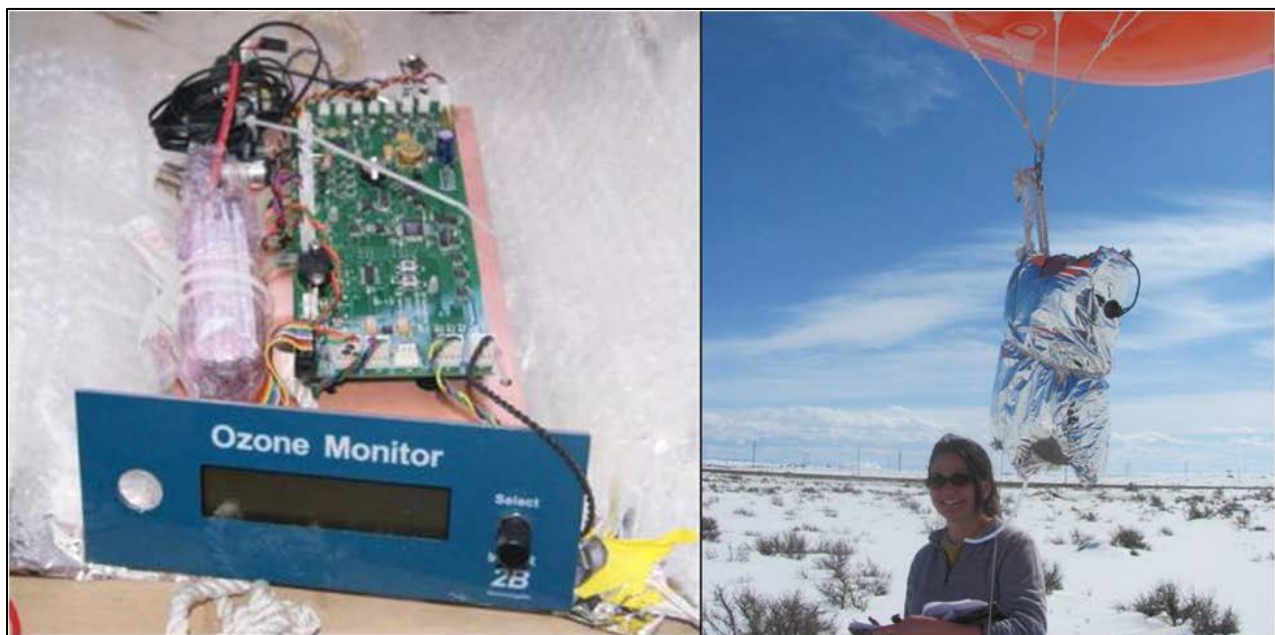
Figure 3-6. Modified 2B Technologies Model 202 ozone monitor remounted to circuit board and deployment at the Red Wash location.
