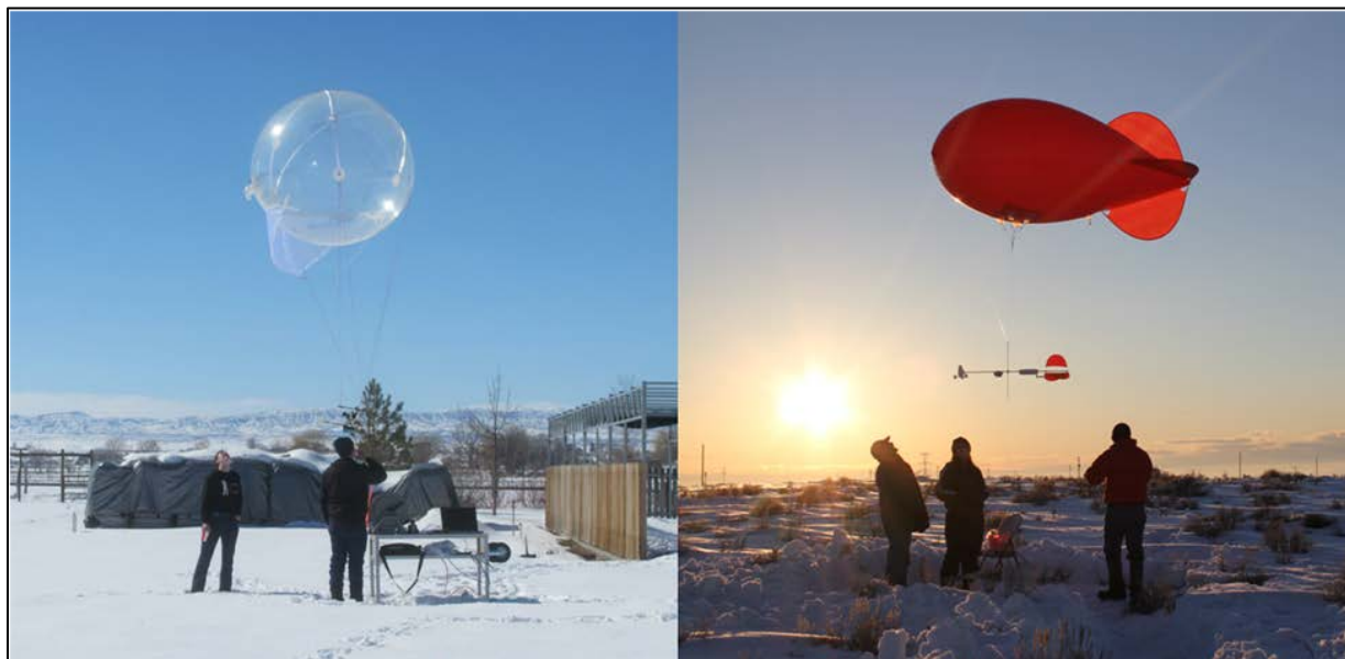
Figure 3-4. Meteorological tethered sonde operations at Jensen (left) and Red Wash (right).
